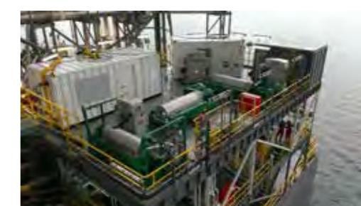
Intergrated Offshore Solids Control/Drilling Waste Management Module
